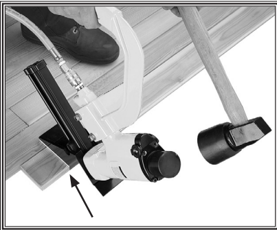
Figure 3. Positioning and operating stapler on flooring strip.
